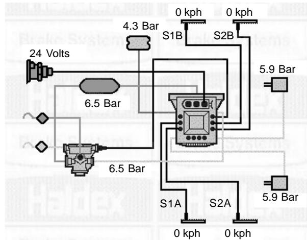
On rotation of the sensed wheels the speed value will be displayed.
