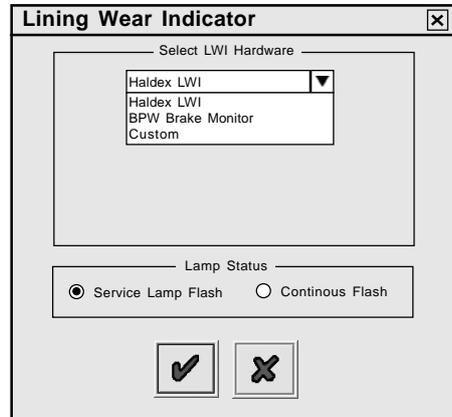
The Custom screen allows the user to enter custom voltage settings as to an alternative manufacturer lining wear system used.
