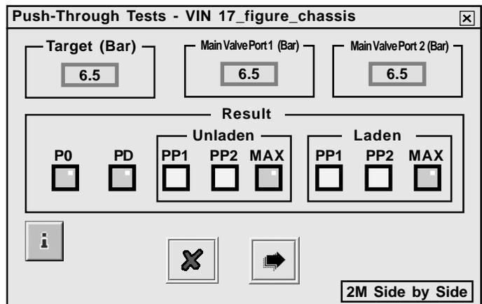
**NB:** Before this test a Warning screen may appear. Make sure that there is the required air pressure in the reservoir to carry out the test. Failure results may occur on the output values (P3) if the value measured (-0.3 bar min.) is below the target value.
