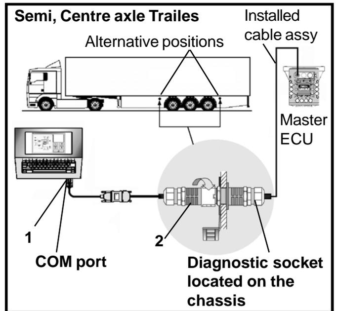
Power the **EB+** system from an external 24V supply and the LED light on the interface pod should now be on, coloured red. If it is not, please check your connections and try again.
