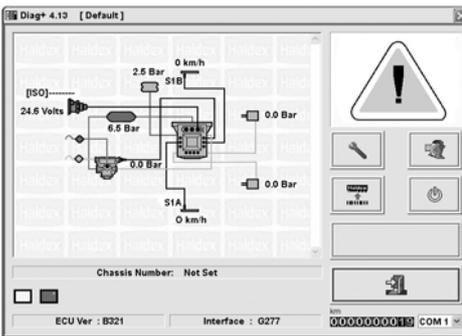
(e) Observe the trailer EBS warning light. The warning lamp should display what has been set in the 'Lamp Setting' section of the ECU Setup.
